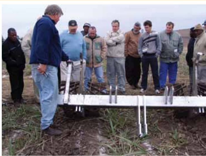
Donald Roseveare turns a ripper on its head to show crumble busters and the adapted spacing of the tines to suit tramline row spacing. The implement was being used to improve water infiltration in the interrow.
