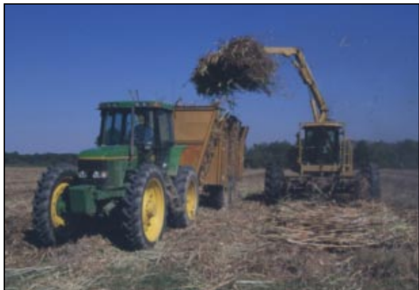
A high capacity slewing push-pile loader in operation.
