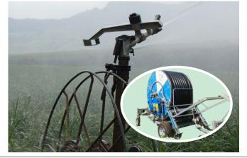
A large sprinkler, namely the Big Gun, is mounted on a trolley/ metal frame and pulled across a field by a cable and winch during an irrigation event. The winch is usually driven by the systems water pressure.
