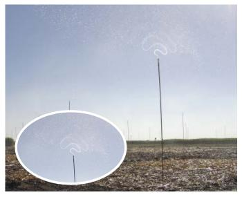
The floppy sprinkler is a uniquely designed light weight sprinkler, consisting of a plastic nipple mounted in a flexible silicone tube. The tube cuts the stream of water into uniform, medium sized water droplets. Over and above the low pressure requirements, each sprinkler is equipped with a flow controller. The floppy system is, typically, a permanent system where spinklers can either be mounted on an overhead cable system or traditional risers.
