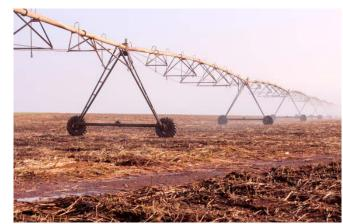
A centre pivot consists of emitters (customised sprinklers) which are mounted onto pipes spanning above the crop. The metal pipes are held together by a metal frame which is supported by 'A' frames on wheels at fixed intervals. One end is fixed at the centre and the remaining structure moves around the centre in a circle.
