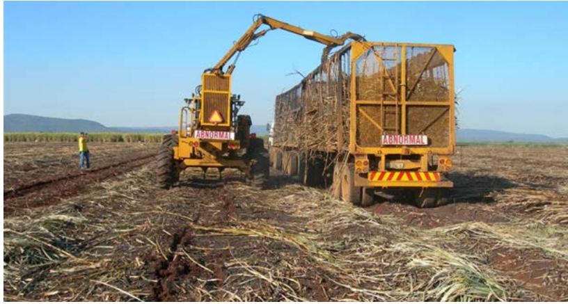
▲ Figure 11: Wheels of all vehicles kept off the crop row in a controlled traffic system.
