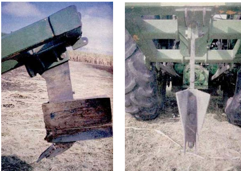
▲ Figure 4: Modification of the ripper tine to incorporate the ameliorant into a vertical slot.
