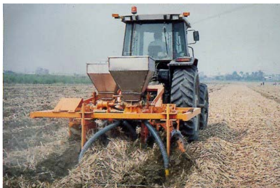
▲ Figure 1: An applicator fitted with a residue coulter and ripper for placing fertiliser in the soil.
