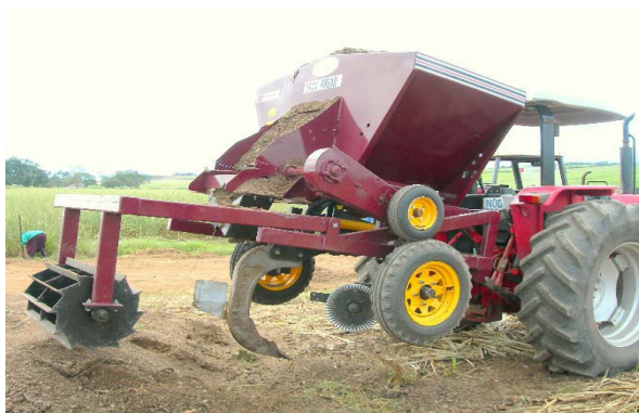
▲ Figure 2: An applicator for chicken litter equipped with a residue coulter, ripper and compactor to level the area worked.
