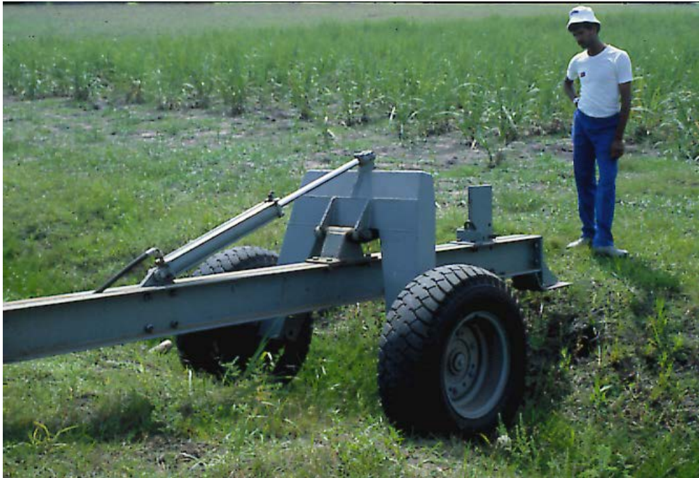
▲ The mole plough in the start position in a ditch.
