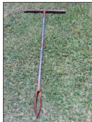
Dutch screw auger.
