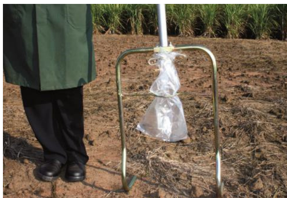
Beater Auger for topsoil fertility sampling ►
