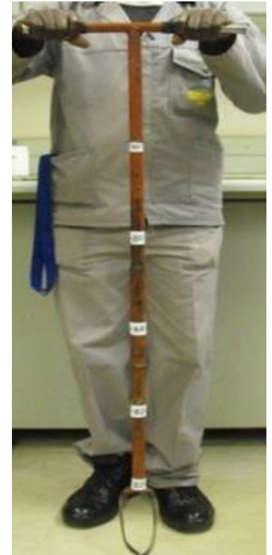
Open bucket (Dutch) auger showing markings to aid sample collection for subsoil acidity or salinity/sodicity sampling. ►
