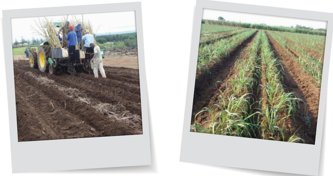
Figure 5a and b: Mechanical planters are available but may need to be modified for the desired traffic zone and cane row spacing configurations.
