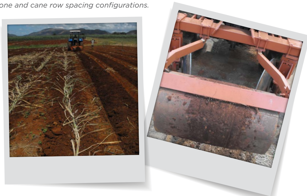
Figure 6a and b: Mechanical furrow closing devices are available and are often used in conjunction with a roller at the back to create a smooth bed (production zone) or field surface. This is an essential requirement for mechanical harvesting operations.
