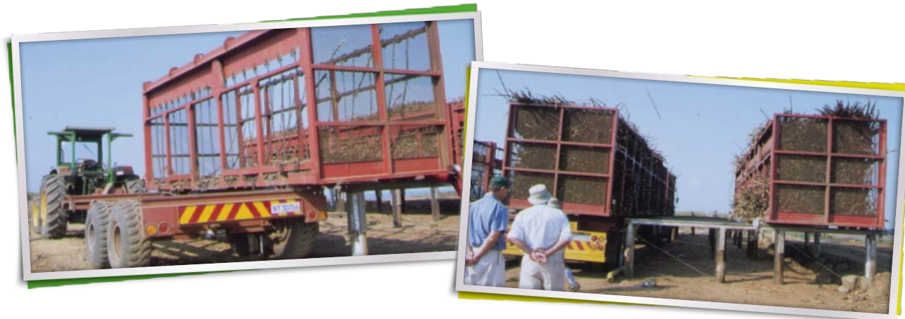
Figure 12a and b: Bin systems are used to minimise infield axle loads and facilitate rapid loading of road haulage vehicles at designated transfer stations. Alternative systems include hook lift systems, high-lift bins or forklift systems for field to road transloading operations.
