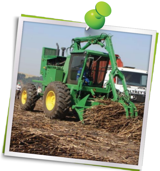
Figure 11: Although slew loaders are typically heavier than non-slew loaders, they are able to constrain infield travel to traffic zones.
