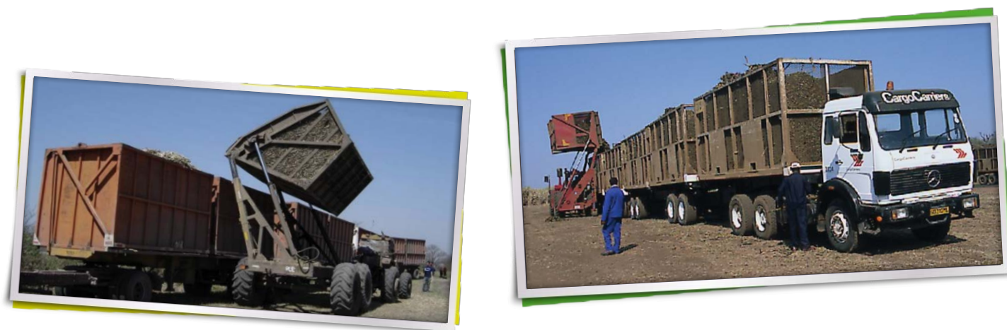
Figure 12a and b: Bin systems are used to minimise infield axle loads and facilitate rapid loading of road haulage vehicles at designated transfer stations. Alternative systems include hook lift systems, high-lift bins or forklift systems for field to road transloading operations.
