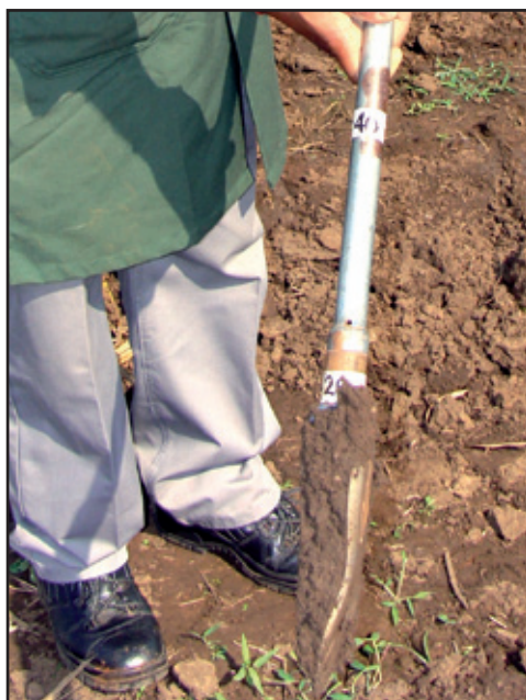
Figure 9.1. Dutch or screw-in auger, used for sampling to depth when subsoil acidity is suspected. The auger should be marked at 20 cm intervals to facilitate depth monitoring of subsamples.
