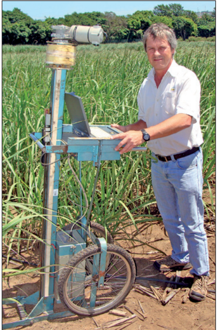
Figure 1.5. A computer driven penetrometer used to detect the severity and depth of compacted layers in soil.
