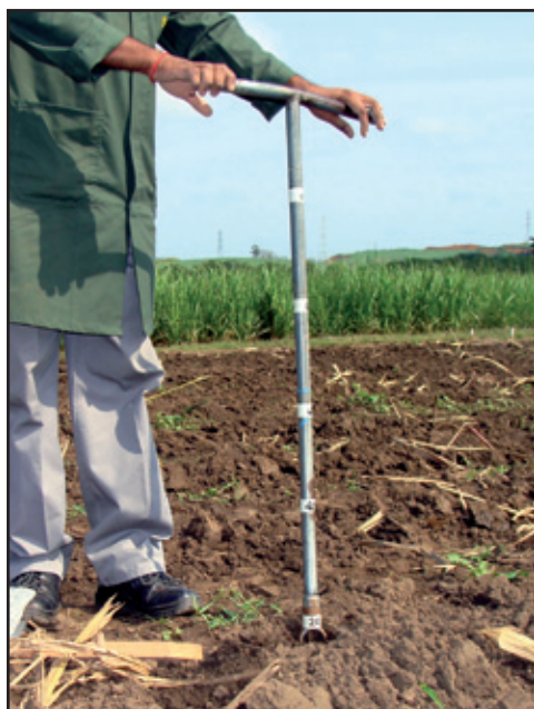
Figure 9.1. Dutch or screw-in auger, used for sampling to depth when subsoil acidity is suspected. The auger should be marked at 20 cm intervals to facilitate depth monitoring of subsamples.
