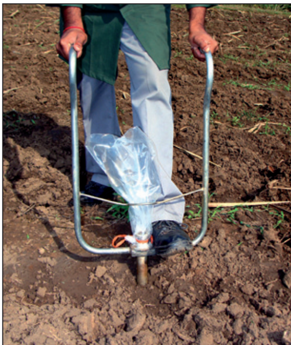
Figure 6.6. The use of the Beater auger for routine soil analyses ensures that a constant sampling depth is maintained.
