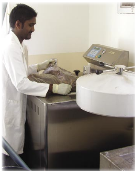
Sterilising facilities in quarantine (such as autoclaves) are used to sterilise soil and plant material.
