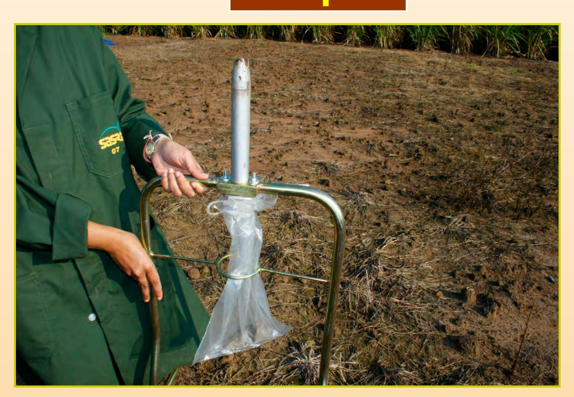
To transfer the core of soil from bit, withdraw the sampler from the ground and invert.
