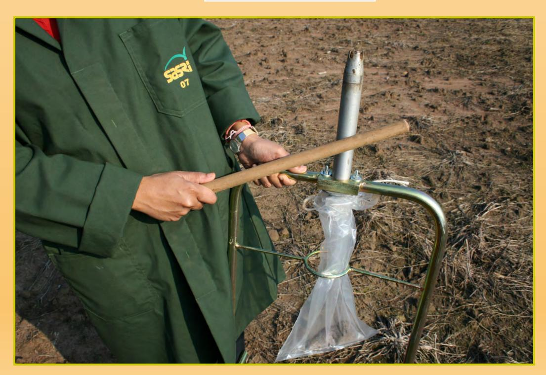
Give the tube a sharp blow with a stick or the butt of the hand to make the core fall into the bag.
