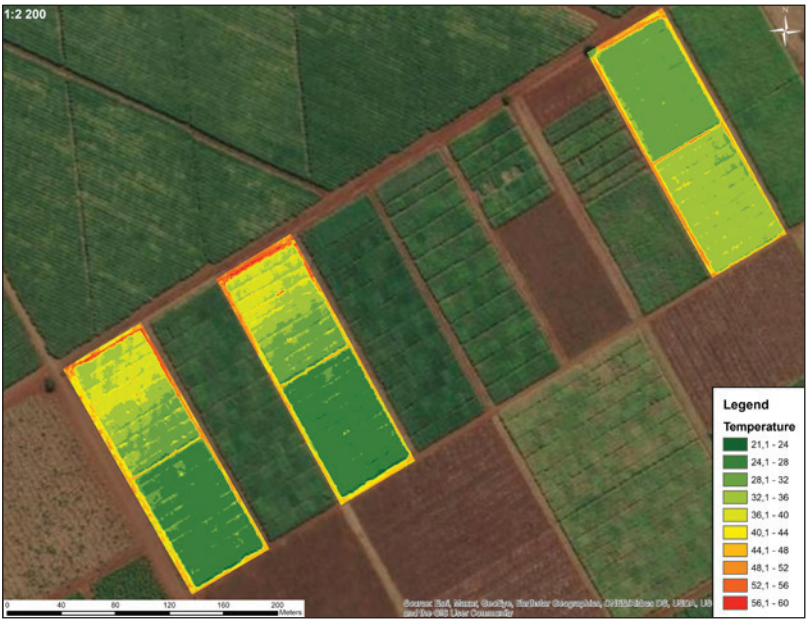
Exploring Aerial Imagery for High-throughput Phenotyping in Breeding. Spectral image obtained by UAV of the SASRI Komati Research Station showing thermal information for three trial replications, each with a well-watered (greenish) and moderately stressed (yellowish) block. Individual plot boundaries are overlaid.
