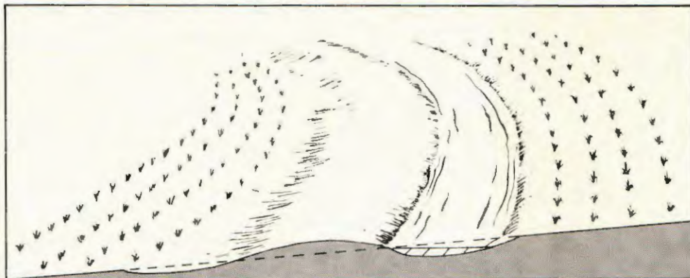
Fig. 1 Retention-type broad based ter- race (slope: up to 10%)
