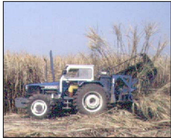
Bundle harvester operating in burnt cane.
