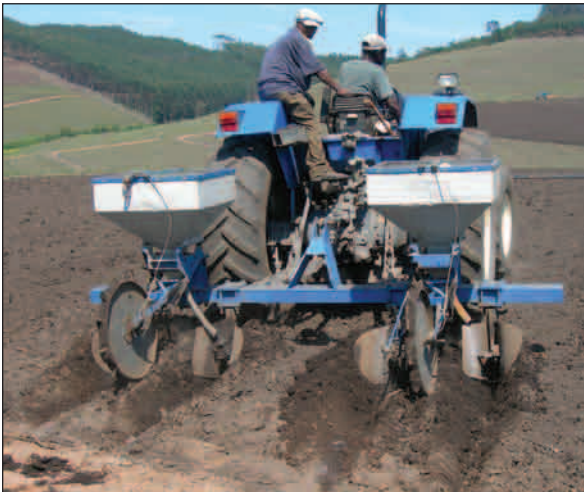
Figure 3. A modified ridger preparing four rows for planting cane in a 1.8 m controlled traffic system.
