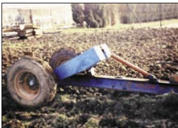
*A mole plough in the operational position – note the long heavy drawbar for stability and evenness of the channel.*
