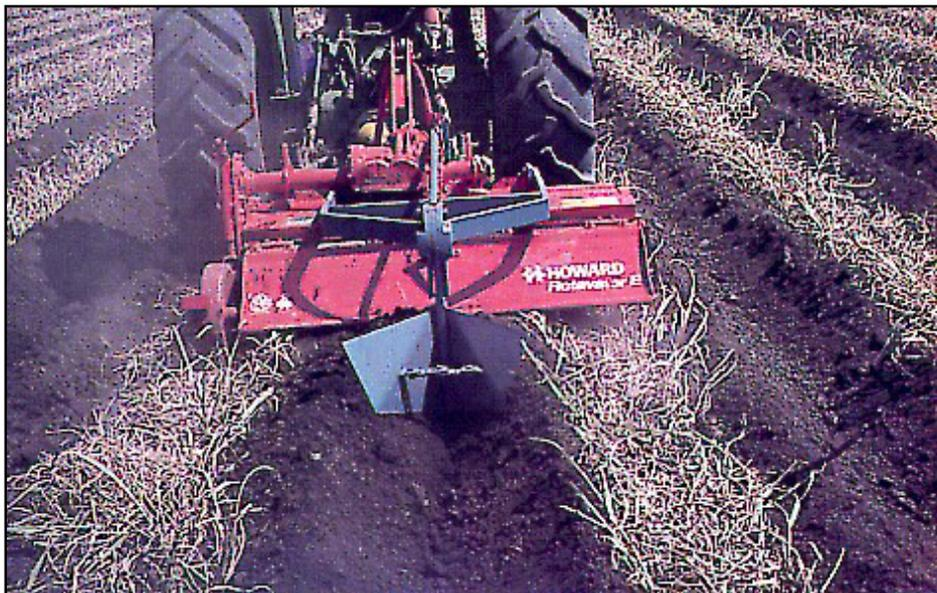
*Minimum tiller in action; limiting cultivation to the old interrow, leaving the dead cane undisturbed.*
