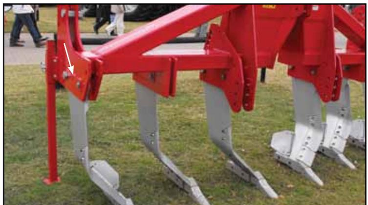
Figure 1. A straight tip subsoiler (left) and a paraplough (right).
