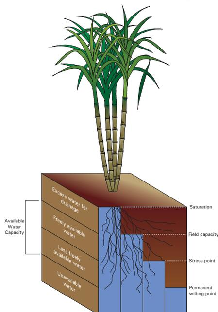
Figure 1 Limits of laboratory-determined soil water content and some relationships between them.
