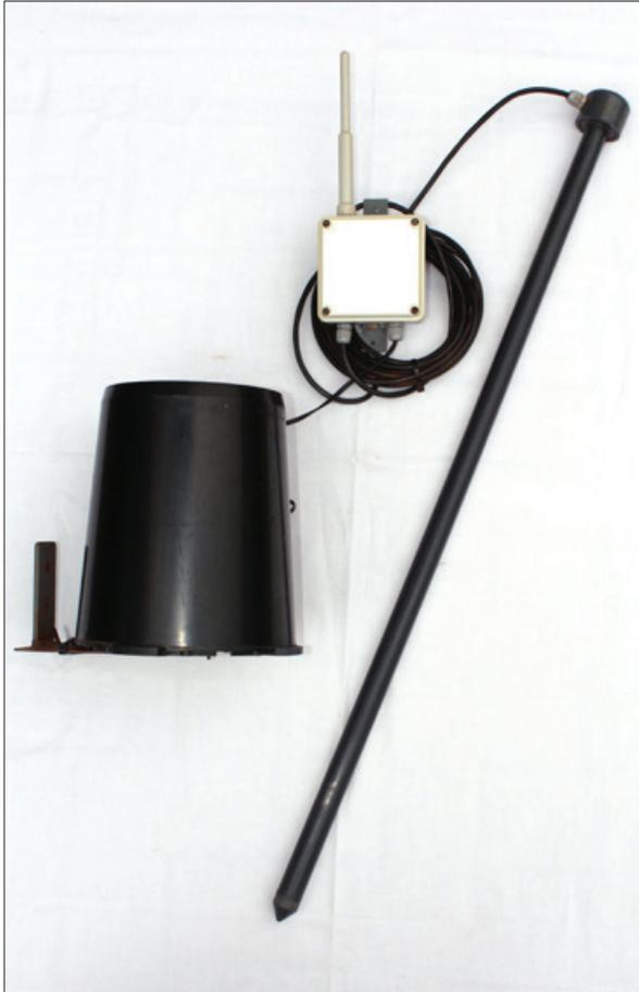
**Figure 2: Capacitance probe**
