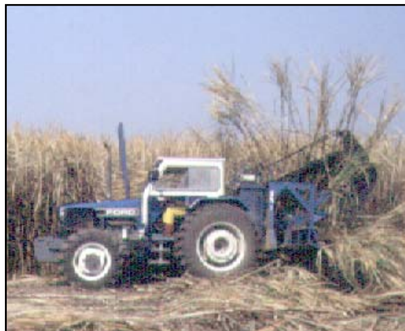
Bundle harvester operating in burnt cane.
