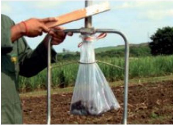
Figure 3. The soil sampler hit with a wooden peg.
