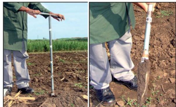
Figure 5. A screw-in (Dutch) auger used to take samples from the subsoil.
