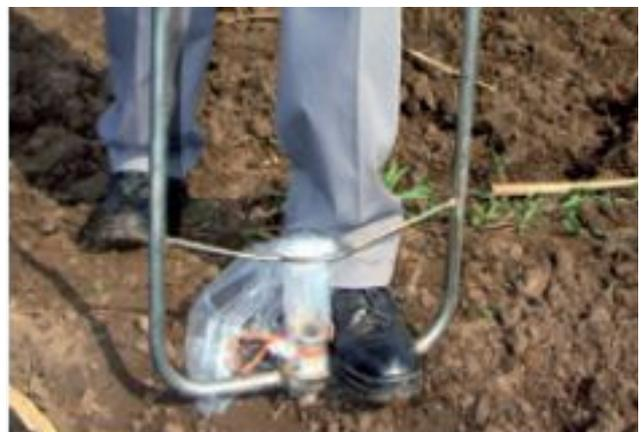
Figure 2. Soil sampler inserted in the soil
