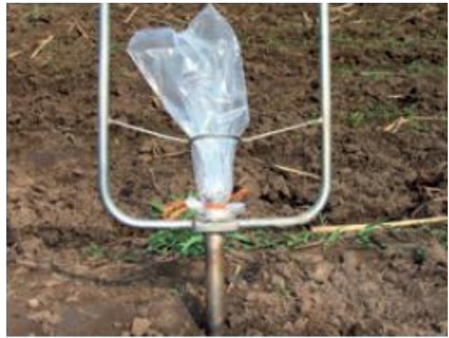
Figure 1. The Beater soil sampler
