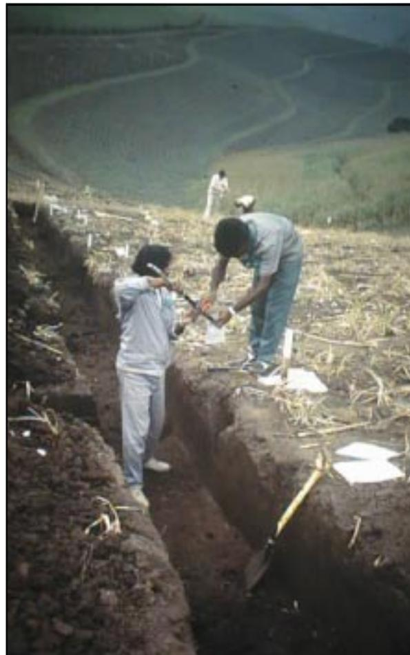
*Figure 3. Trench used for measuring volume and depth of soil disturbance.*
