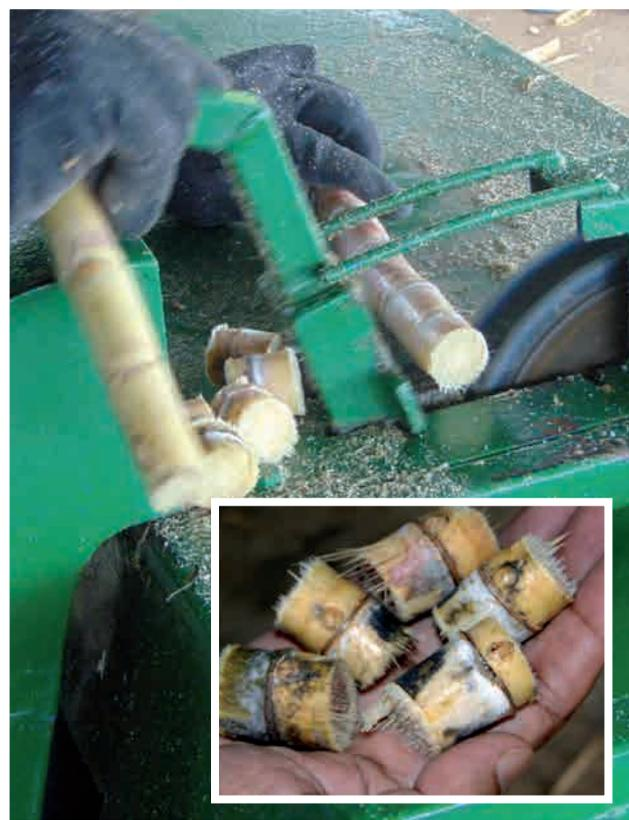
**Single budded setts are prepared using a twin blade circular saw.**
