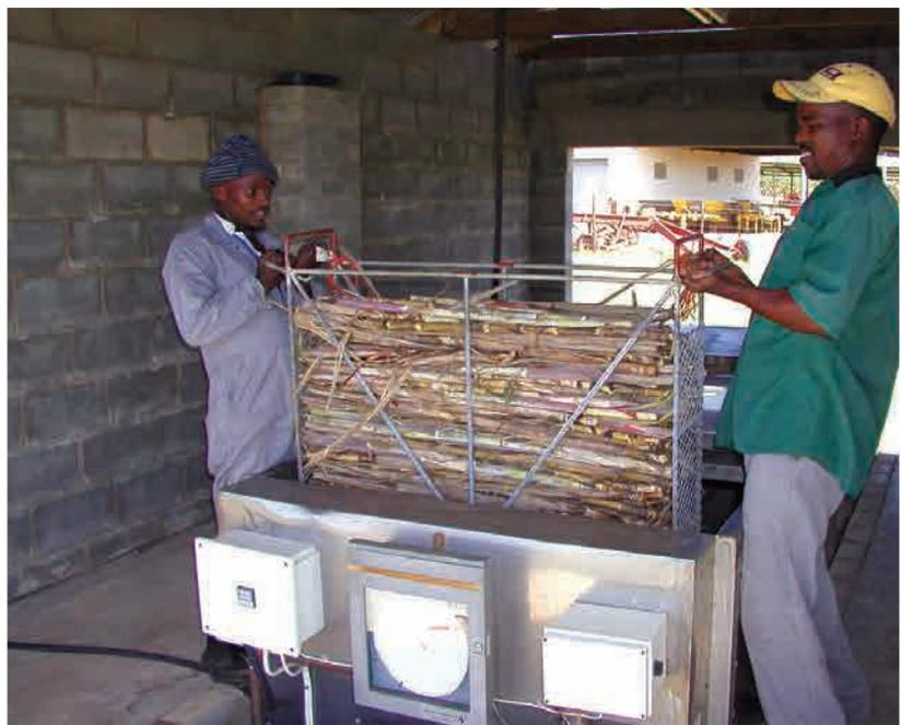
**Seedcane being lowered into an Upfold hot water treatment tank.**
