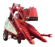
The INTA harvester is a prototype design being researched and developed in Argentina. It has been developed to cut and load whole stick green cane into an accompanying trailer. It is not yet commercially available.
