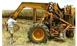
• Ngwenya: This machine was developed as a green cane soldier type harvester which would cut, top, detrash and bundle between 200-300kg of green cane.
