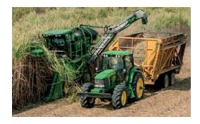
Chopper harvesters have however met most of the requirements of harvesting under a larger range of conditions, slopes, lodged cane, green cane, and topping requirements.Due to their high costs, mechanical harvesters require a large throughput to make them cost effective. The extraction vehicles that support the harvester also need to be taken into consideration. Mechanical harvesting systems also require infield
