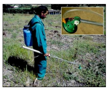
Typical gravity fed CDA system. Insert: spinning disc applicator.
