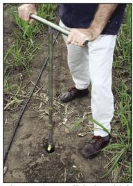
Observation well hole which phas been augered using a Dutch screw auger.
