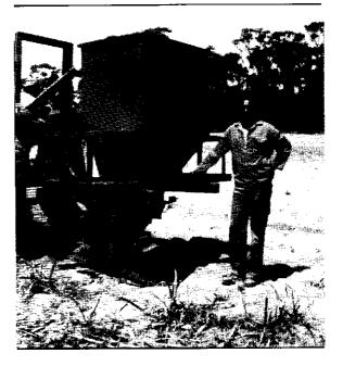
pulled through the banded material. Alternatively, a hopper can be fitted onto the toolbar of the vertical mulcher and the ameliorant fed through a 200 mm diameter downpipe directly behind the tine and into the open slot.
