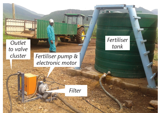
Figure 2. Examples of fixed and mobile active chemical injection systems.
