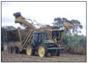
A fully mechanised green cane chopper harvester in operation.
