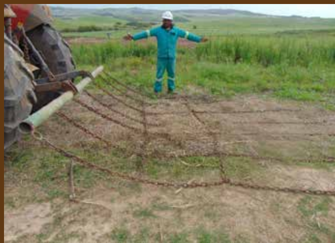
Chain lattice attached to the tractor
